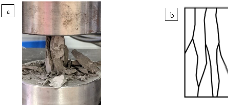
Figure 7. a) Cement cast failed in the UTM machine b) Type 3 columnar vertical cracking
